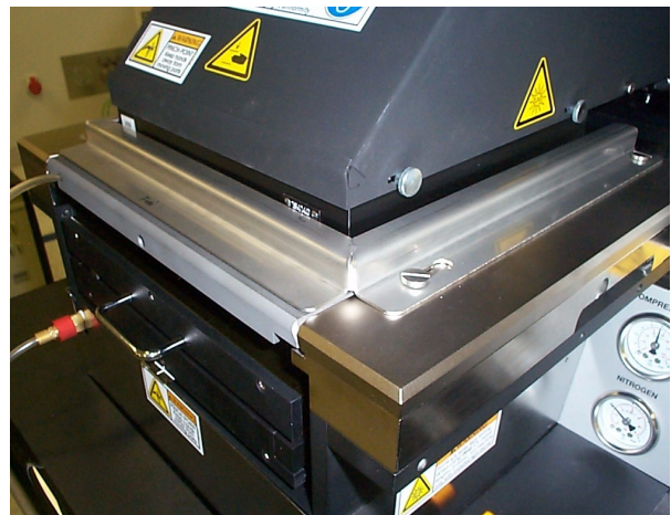
Picture shows special cover for deep-UV exposures
