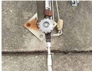
6. Close the small valve when LN2 begins to flow from the end of the fill line.
