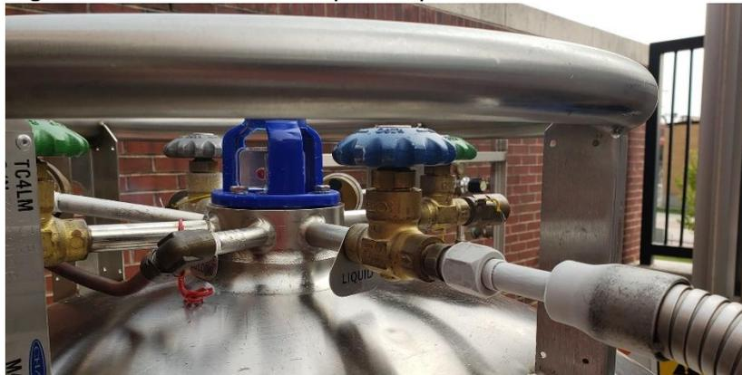
9. Open the vent valve on the dewar. Make sure the vent is pointed to the brick wall.
