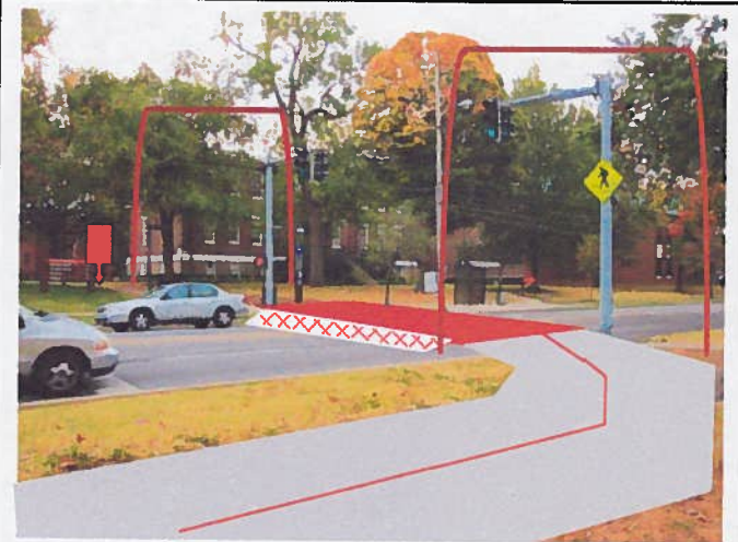
Raised table mixed-use path crossing; Library south. Library Loop and West Campus Gateway locations.
