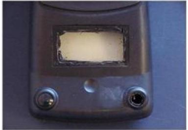
2. Staff should also be aware of the addition of keypad overlays. An overlay can be a small sticker that forms to the device and covers the keyboard area. Overlays may hide damage due to tampering or wires that can allow for keyboard logging. Overlays should not be used.
