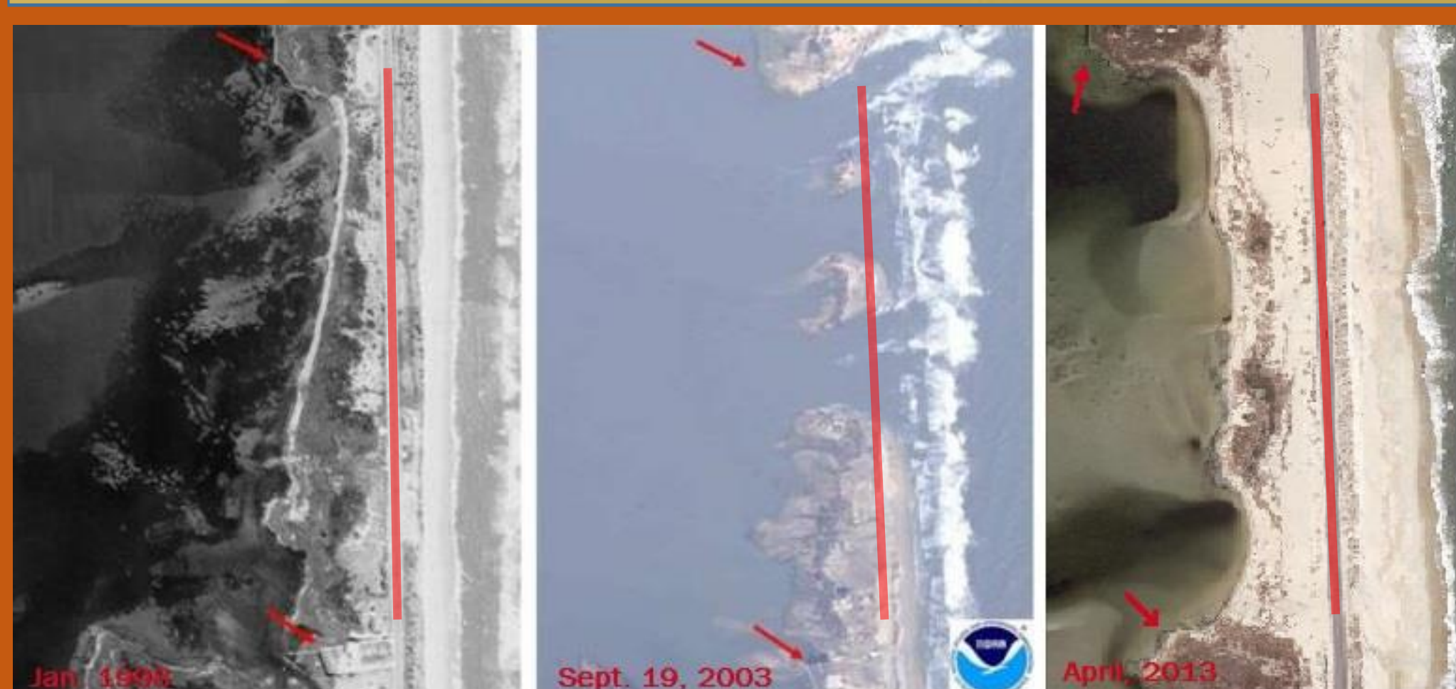
Aerial photos of Cape Hatteras seashore before Hurricane Isabel (left), just afterward with the road missing (middle), and 10 years later with the road repaired (right). Red arrows point to corresponding locations. The road, Highway 12 (red line), was the only access to mainland for the ~200 residents of Hatteras Village, NC. Images courtesy NOAA Report "Hurricane Isabel Damage Assessment at Cape Hatteras" and Google Earth.
