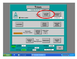
From here we can either load up an old recipe or create a new one. To load a previous recipe hit the "**Recipe from Disk**" button and choose the proper recipe from the list and verify that it has the intended parameters. The recipe files are stored in **C://Trion/recipes** if they ever need to be retrieved. Once you are satisfied with the recipe select exit to load it on to the metal etcher.
