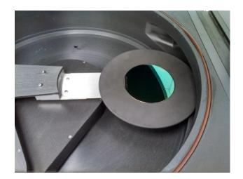
The loadlock will now pump down so that it can transfer to process chamber. Press **OK** when prompted by the software. You are ready to continue processing if the Loaded icon turns green.
