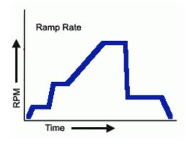
In addition to spin speed, acceleration can also affect the coated film properties. Since the resin begins to dry during the first part of the spin cycle, it is important to accurately control acceleration. In some processes, 50% of the solvents in the resin will be lost to evaporation in the first few seconds of the process.
