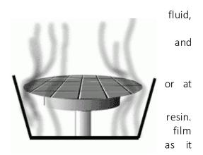
process. This can lead to radial thickness non-uniformities since the fluid viscosity changes with distance from the center of the substrate. By slowing the rate of drying, it is possible for the viscosity to remain more constant across the substrate.
