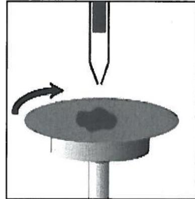
One of the most important factors in spin coating is repeatability. Subtle variations in the parameters that define the spin process can result in drastic variations in the coated film. The following is an explanation of some of the effects of these variations.
