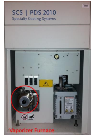
Figure 4 Vaporizer location for loading monomer
