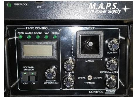
Figure 1 TT-3/6 E-beam power supply controller panel
