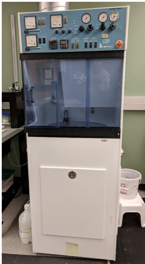
Figure 3. The donated Logitech CCP mechanical polishing system installed in the packaging lab of the MNTC.
