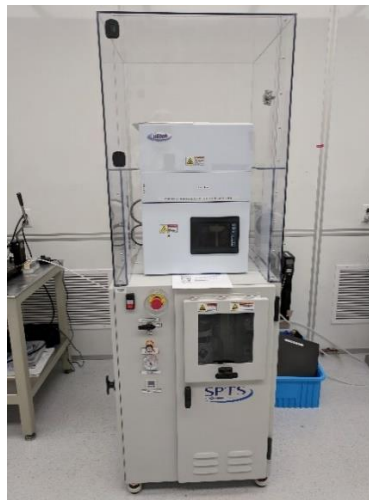
Figure 2. The newly installed SPTS etch system that can perform etching with hydrofluoric acid in a vapor form.
