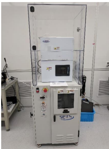
Figure 2. The newly installed SPTS \mu etch system that can perform etching with hydrofluoric acid in a vapor form.
