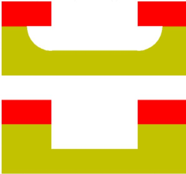
Etching can be **isotropic**, i.e., exhibiting a lateral undercut rate on a patterned surface approximately the same as its downward etch rate.
