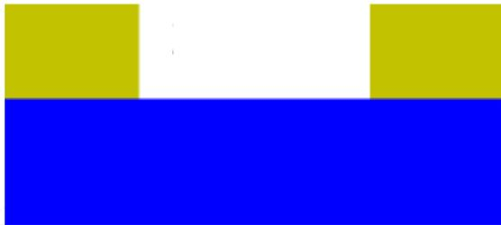
$$\text{Selectivity} = \text{Etch Rate A} / \text{Etch Rate B}$$
