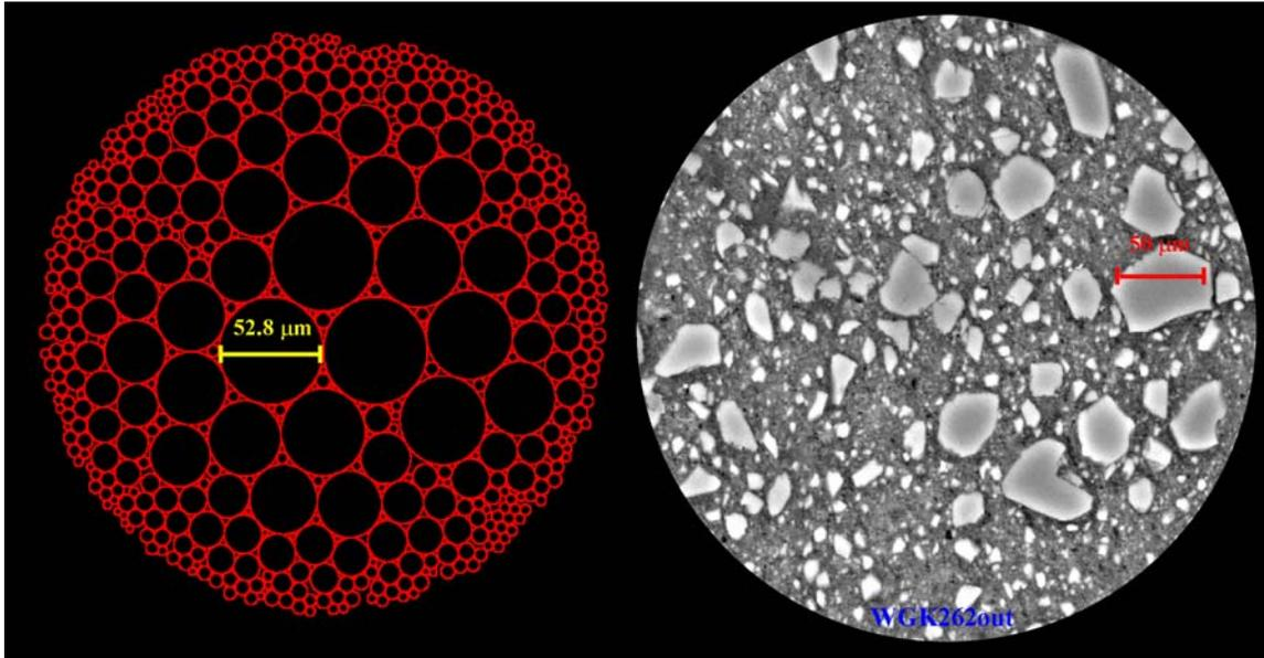
Typical simulated texture based on pooled particle size distribution data from 3 telescopic SEM images (1K, 2K, and 4K magnifications). Only the 1K image is shown.  $N = 528$  particles.
