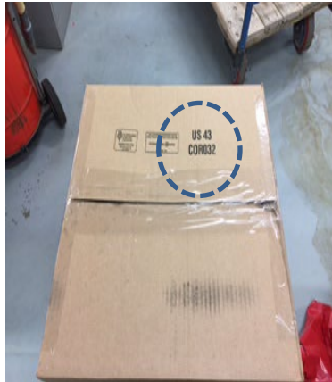
STEP 2: Fold bottom flaps down, DoT spec mark visible (US 43). Use 2" wide clear tape to securely tape the middle seam (at least 2 strips) .
