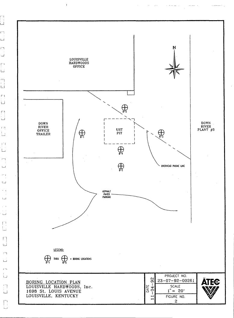
On October 16, 1992, ATEC advanced five (5) soil borings adjacent to the former UST pit using a truck-mounted rotary drill rig equipped with 3-3/8 inch I.D. hollow stem augers. Soil samples were collected at 5.0 ft intervals using carbon steel split-spoon samplers. The location of each boring, is displayed on Figure 2.
