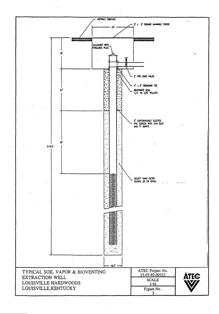
proposed location of the soil bioventing system will be centered around the former UST installation pit and will utilize several of the existing monitoring wells. A vacuum will be placed on the extraction points to induce volatilization, removal of subsurface volatiles, and oxygen transfer. An enclosure blower unit will be used to supply the vacuum source.
