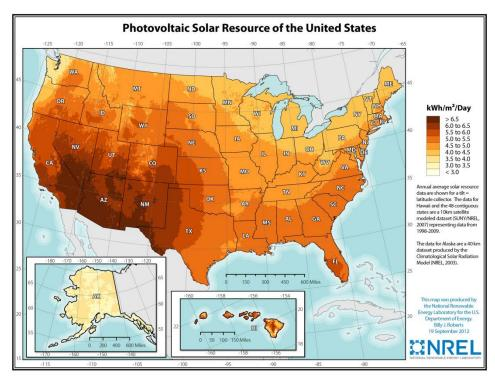
Figure 2: Solar Resource Map USA<sup>2</sup> Source: NREL
