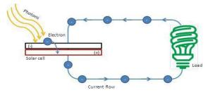
Figure 8. Generation of electricity from a PV cell Source: NREL
