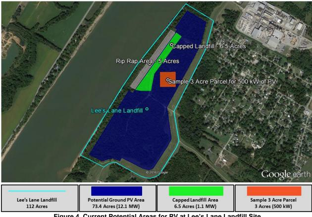
Figure 4. Current Potential Areas for PV at Lee's Lane Landfill Site Source: Google Earth
