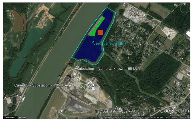
Figure 7. Utility Substations Near Lee's Lane Landfill (Photo Credit: Google Earth)
