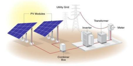
Figure 1. Ground Mount PV Array Source: NREL
