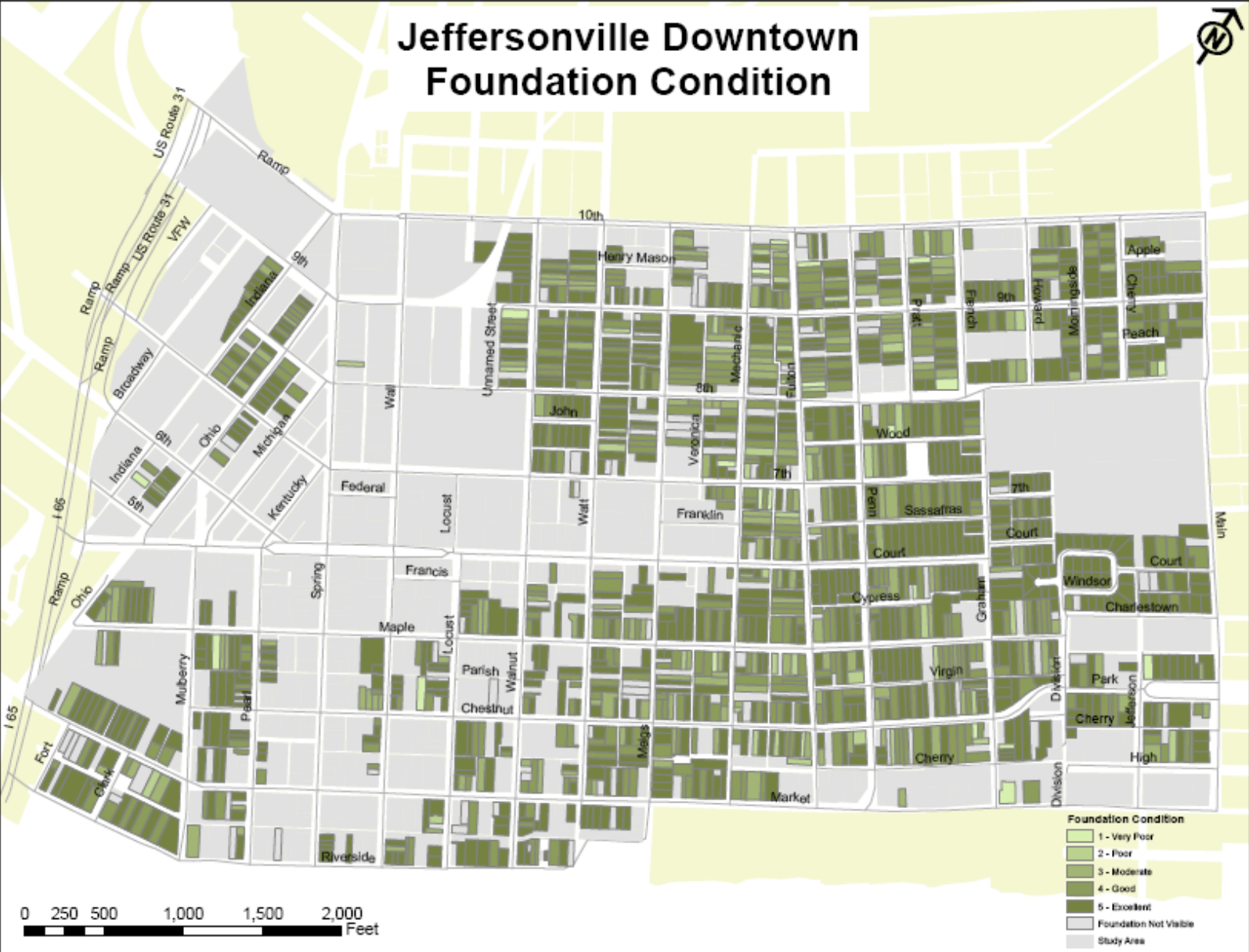
Map 16: Individual Property Foundation Condition
