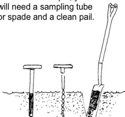
**3** Sample to proper depth. If a spade is used, dig a V-shaped hole to the depth of sample. Obtain a slice or core of soil from the surface of the ground, downward to the appropriate depth as listed below. Use a spade to cut a thin slice of soil. First, push the spade into the soil and throw this soil aside. Take a one-inch thick slice of soil from the back of the hole at the proper depth.
