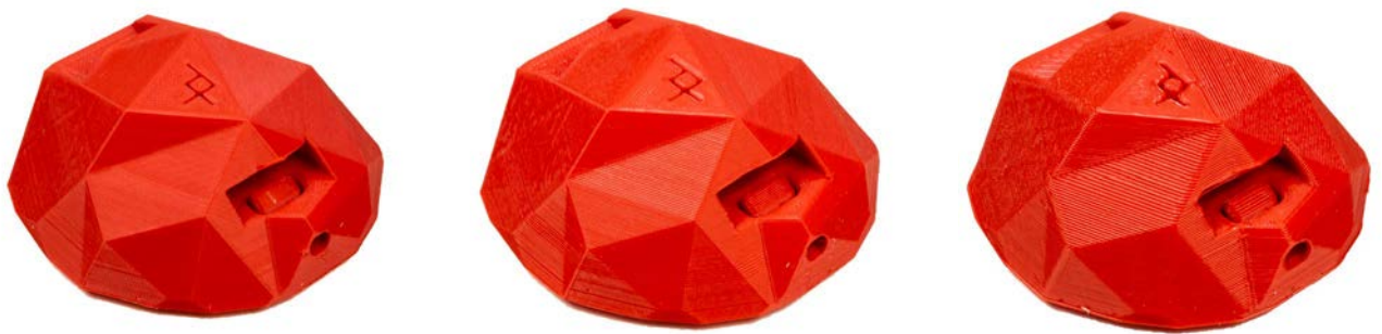
Three examples printed at different layer heights (left: 0.1 mm, center: 0.2 mm, right: 0.3 mm). Model credit: print+
