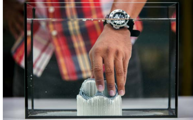
PVA (the white material) dissolves away from the model in water
