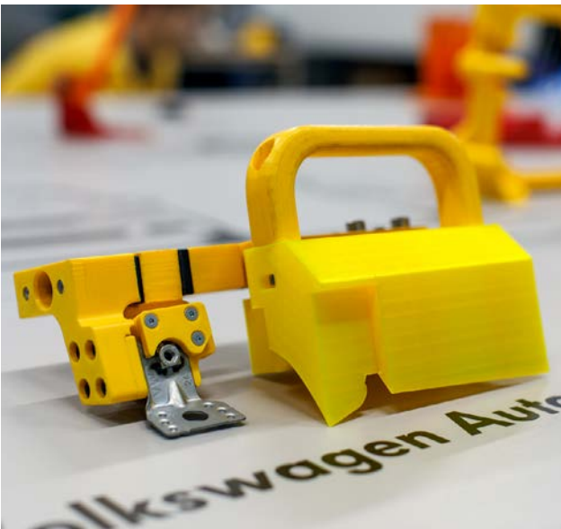
A 3D printed tool assembled from multiple parts
