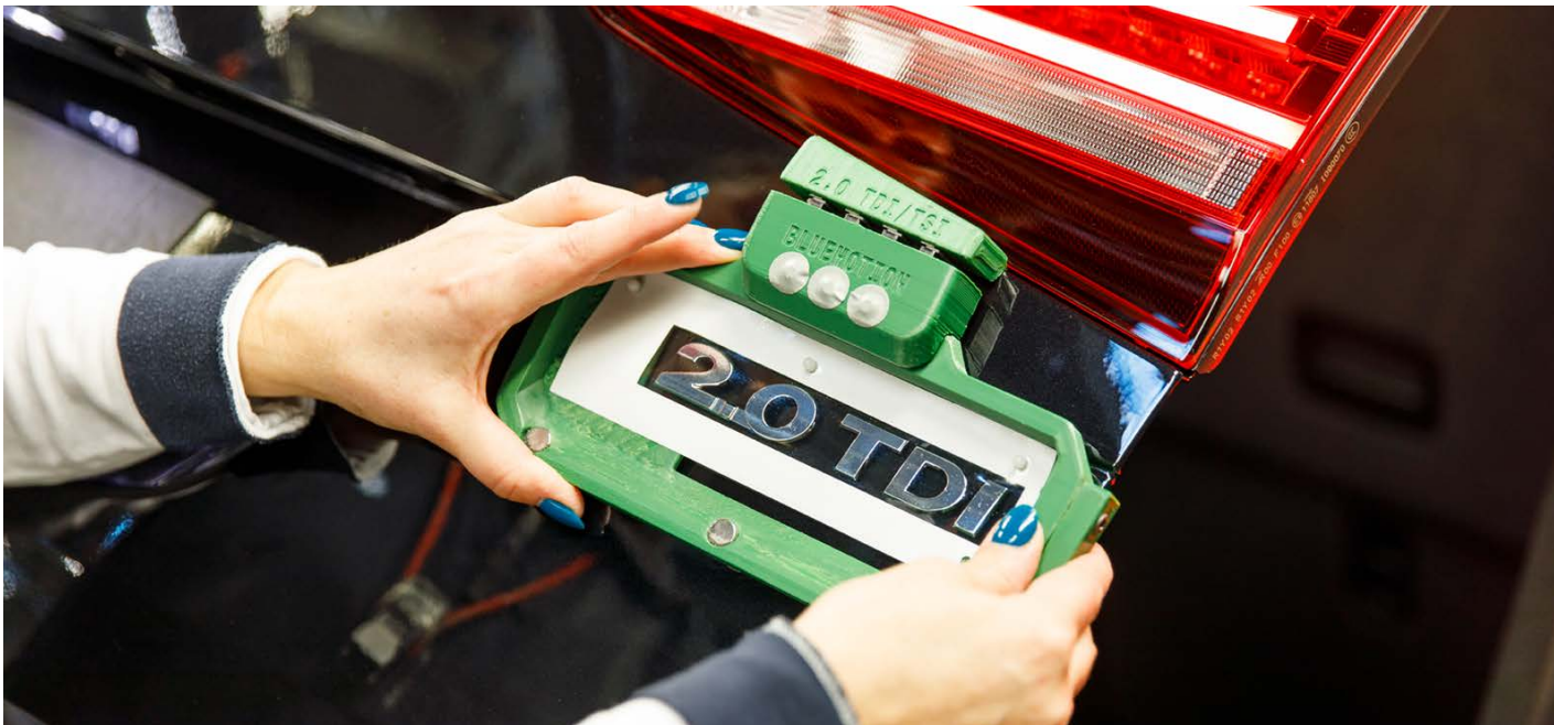
Volkswagen Autoeuropa use Ultimaker printers to create tooling for the production line
