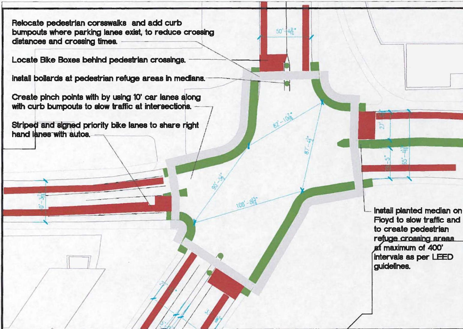
Relocate pedestrian crosswalks and add curb bumpouts where parking lanes exist, to reduce crossing distances and crossing times.
