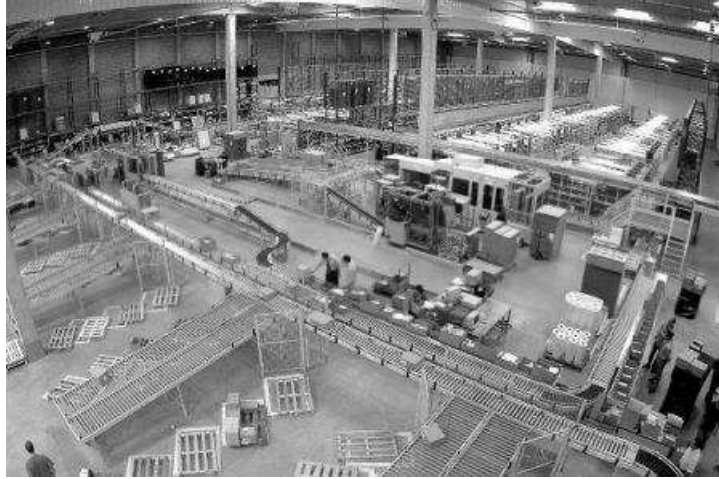
Figure 1.1. An integrated warehouse MH system
