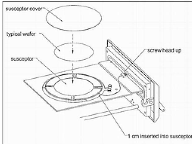
**Figure 3.** Susceptor installation and sample placement.
