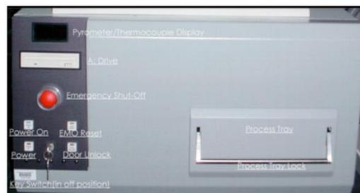
Figure 1. Front panel of the RTP.
