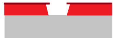
The result should hopefully be that the toluene overhangs over all your features giving you the separation between the thin films. It is worth noting while this method is the most difficult, it also tends to effect the sizes of features since the Toluene overhangs the edge of the photoresist.
