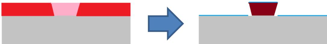
**Liftoff using LOR3A** is also very commonly performed in the cleanroom. This technique involves pre-coating the wafer with a chemical that etches slightly faster than photoresist in developer. This should result in a photoresist profile that looks “undercut” and allows a gap between the thin film on the wafer with what is on the photoresist.
