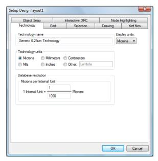
This window allows us to select exactly how the drawing is going to be scaled. This is important in order to prevent your 10 microns feature from ending up a 10 millimeter feature. For all files being sent to KORE, the window above shows the optimal settings. The "technology units" should be set to microns and one internal unit should be equal to a thousandth of a micron. This internal unit shows the smallest amount of resolution in which the software can operate.
