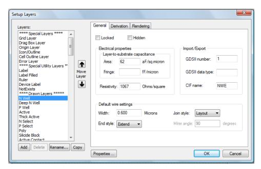
When exporting to a GDSII format, the names of the layers are lost. Instead each layer is defined by the "GDSII number" seen in this window. Therefore it is important to ensure that each layer used has a uniquely defined GDSII number and all mask instructions reference this number. The numerical value itself is not important to the mask, so it can be arbitrarily assigned so that it is uniquely defined from all other layers drawn in the file. Choose any unique number from 1 to 100 for each layer.
