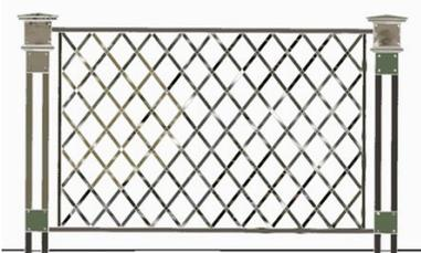
**Figure 93:** Drawing of existing railing on the unused automobile lanes on the east and west side of the K&I Bridge.
